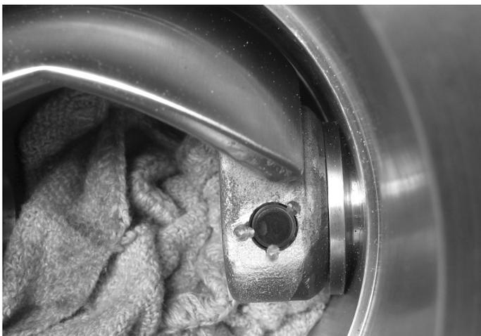
**Figure 41** 1 to 2 Inch Shaft Connection Stake Example
