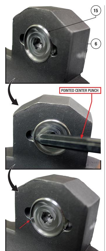
Figure 57 16 to 24" NPS Shaft Retainer Stake Detail
