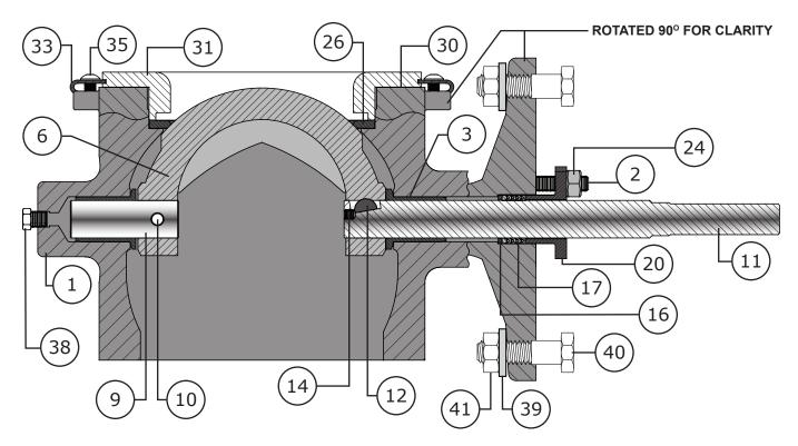
Figure 77 3 to 8" NPS (80 to 200 DN) Model 570 Cross Section
