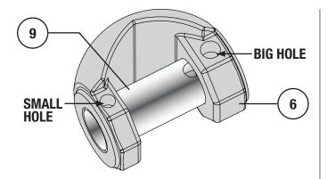
Figure 39 1 & 1-1/2" NPS Follower Shaft Installation
