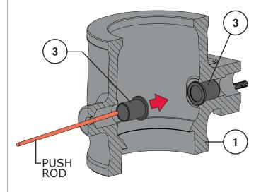
Figure 33 3 to 12" NPS Outboard Bearing Removal
