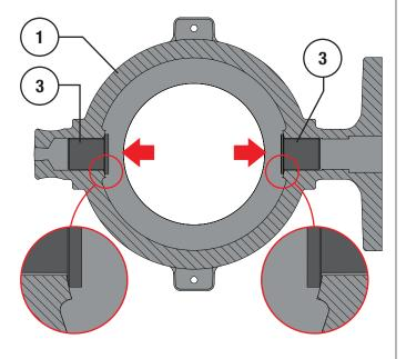
Figure 37 Bearing Placement in Valve Body
