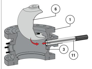
Figure 50 16 to 24" NPS Drive Shaft / Ball Installation
