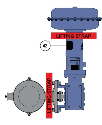
Figure 2 Actuator Lifting Strap Placement Suggestion
