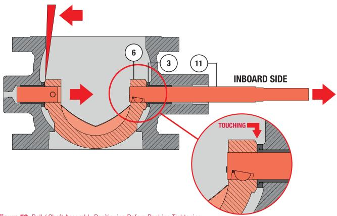
Figure 59 Ball / Shaft Assembly Positioning Before Packing Tightening
