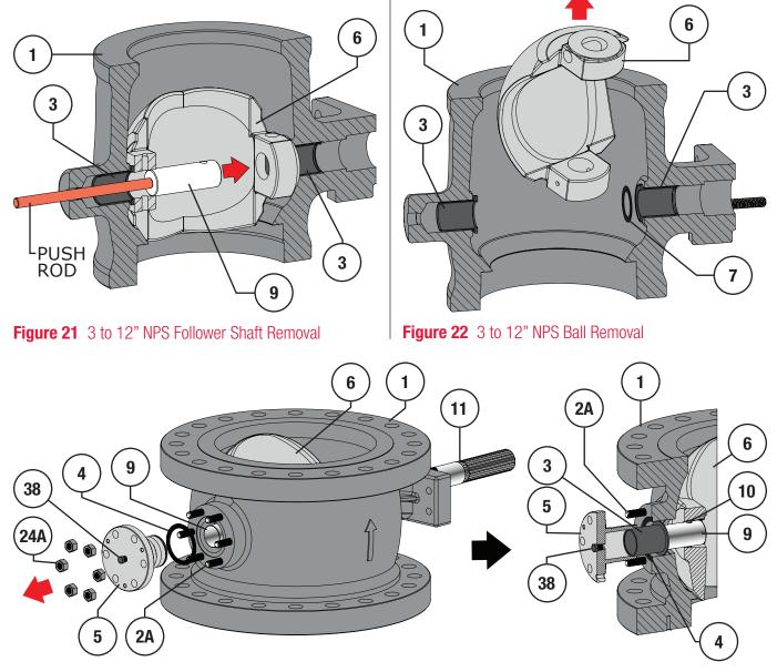
Figure 23 16 to 24" NPS (400 to 600 DN) Flange / Spiral Wound Gasket / Bearing Removal
