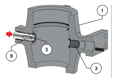
Figure 44 1 to 4, 10 & 12" NPS Follower Shaft Installation
