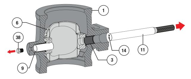
Figure 20 3 to 12" NPS (80 to 300 DN) Drive Shaft / Pipe Plug Removal
