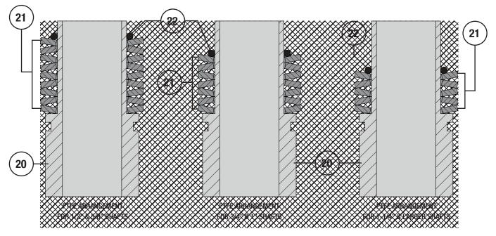
Figure 63 Live-Loaded PTFE Spring Washer Arrangements
