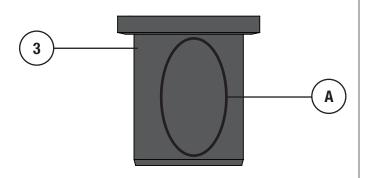
Figure 36 Anti-Seize Application to Bearing
