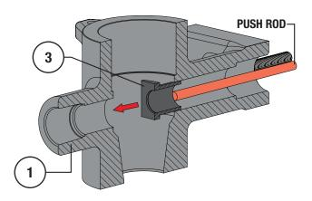
Figure 32 1 to 2" NPS Inboard Bearing Removal
