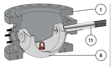
**Figure 51** 16 to 24" NPS Drive Shaft / Ball Installation (Step 2)
