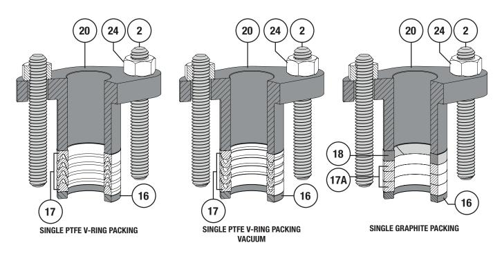
Figure 60 Standard Packing Configuration Diagrams
