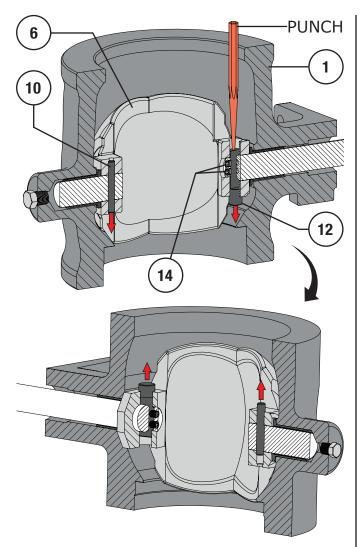
Figure 19 3 to 12" NPS Shaft Connection Disassembly
