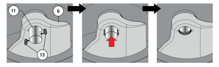
Figure 53 16 to 24" NPS Drive Shaft Pins Installation Sequence
