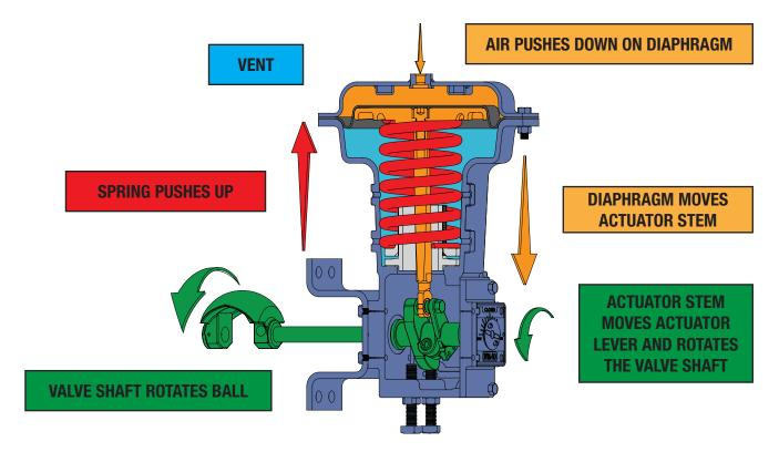
Figure 8 Principles of Operation - Actuator & Valve Mechanics
