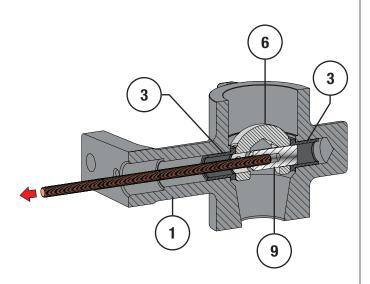
**Figure 18** 1 & 1-1/2" NPS Follower Shaft Removal (Obsolete Valve Body Design)
