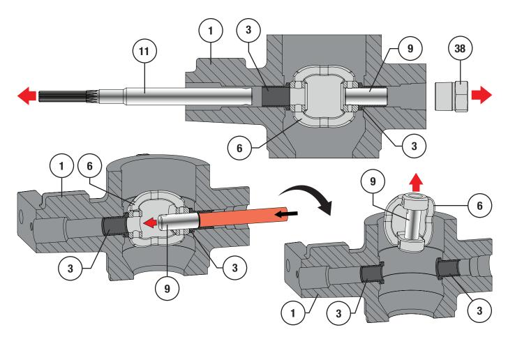
Figure 17 Follower Shaft and Ball Removal (Steps 6 to 10 for 1 to 2" NPS Valves)
