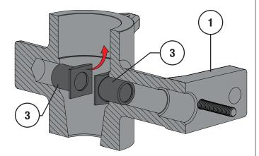
**Figure 31** Old Style1 & 1-1/2" NPS Bearing Removal (Obsolete Valve Body Design)
