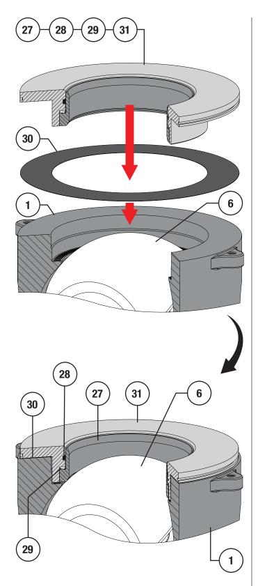
Figure 69 Metal Ball Seal Installation
