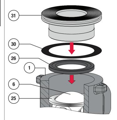
Figure 65 1 to 2" NPS Ball Seal Installation
