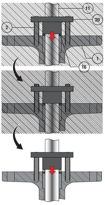
Figure 58 Packing Ring Installation Detail
