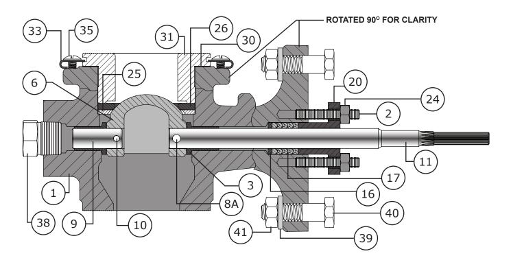
Figure 76 1 to 2" NPS (50 DN) Model 570 Cross Section
