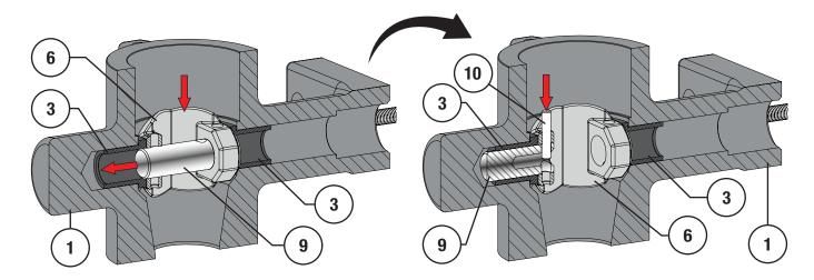
Figure 40 1 to 2" NPS Ball / Follower Shaft Installation (Obsolete Valve Body Style Shown)
