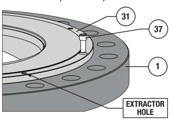
Figure 11 Seal Protector Ring Retaining Parts Removal
