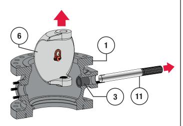
Figure 29 16 to 24" NPS Ball/Follower Shaft Removal
