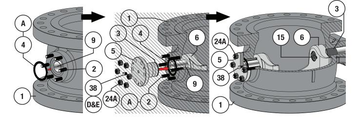
Figure 56 16 to 24" NPS Spiral Wound Gasket and Flange Assembly Installation Sequence
