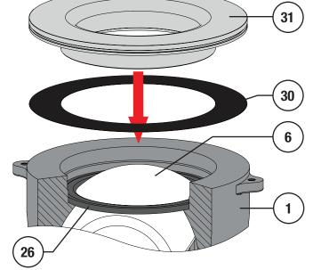
Figure 66 3 to 24" NPS Ball Seal Installation
