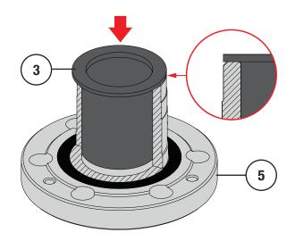
Figure 38 16 to 24" NPS (400 to 600 DN) Outboard Bearing Installation
