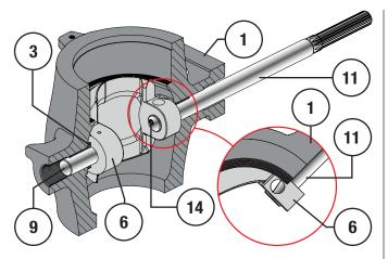
Figure 48 3 to 12" NPS Drive Shaft Installation
