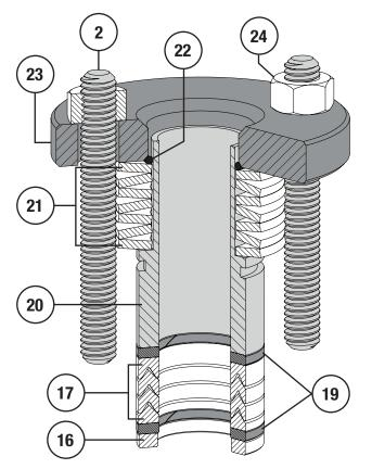
**Figure 61** Live-Loaded PTFE Packing Ring Installation Detail (Refer to Figure 63 for Spring Washer (Key 21) Arrangements
