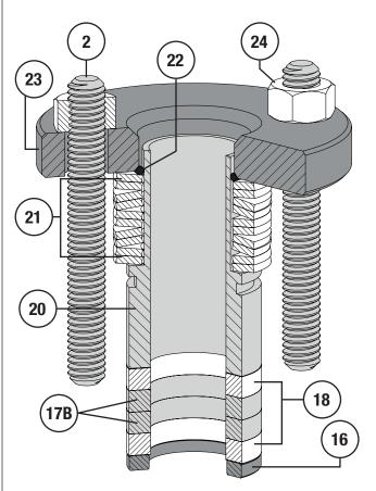
**Figure 62** Live-Loaded Graphite Packing Ring Installation Detail (Refer to Figures 62 for Spring Washer (Key 21) Arrangements
