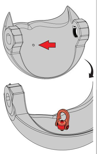
Figure 26 16 to 24" NPS Ball Lifting Hook Placement
