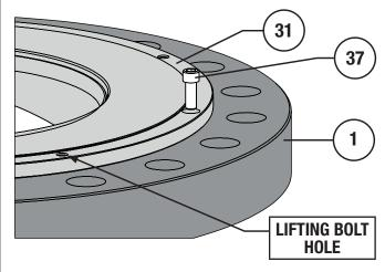
Figure 67 Seal Protector Ring Retaining Parts Installation
