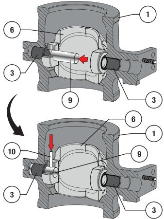
Figure 46 6 & 8" NPS Follower Shaft & Pin Installation
