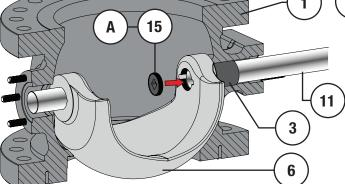
Figure 55 16 to 24" NPS Shaft Retainers Installation
