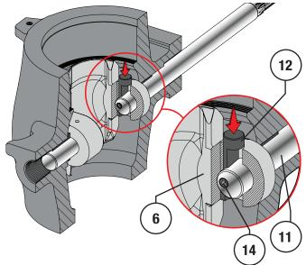
Figure 49 3 to 12" NPS Shaft Key Installation
