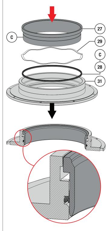
Figure 68 Metal Ball Seal Assembly
