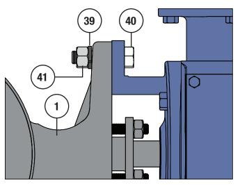
Figure 7 Actuator Mounting Detail
