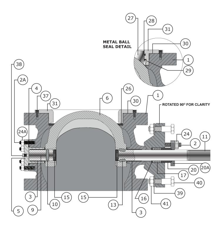
Figure 79 16 to 24" NPS (400 to 600 DN) Model 571 & 573 Cross Section
