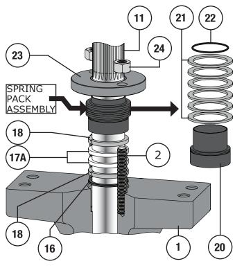
Figure 10 Sample Live Loaded Packing Removal
