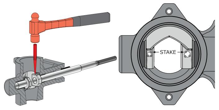
**Figure 42** 1 to 2" NPS Shaft Connection Pin Stake Locations (2" NPS valves are staked on opposite sides of the ball from each other)
