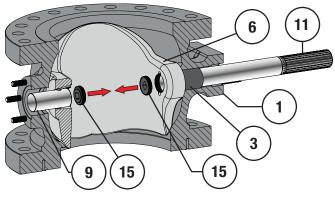
Figure 24 16 to 24" NPS Shaft Retainer Removal
