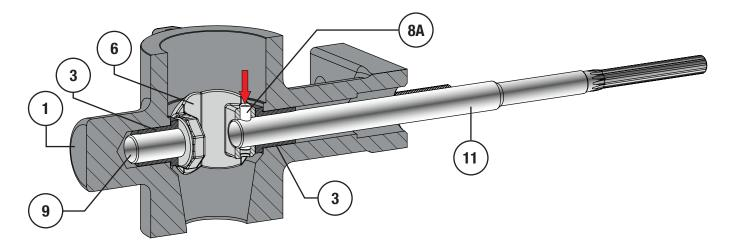
Figure 41 1 to 2" NPS Drive Shaft Installation (Obsolete Valve Body Design Shown)
