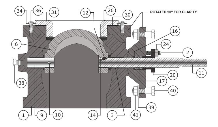
Figure 78 3 to 12" NPS (80 to 300 DN) Model 571 & 573 Cross Section
