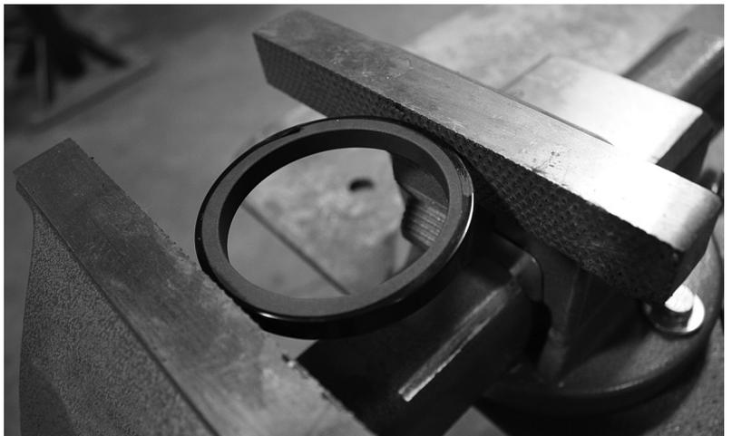
**Figure 24** Model 351 Piston Ring Vise Break Method (Step 2)
