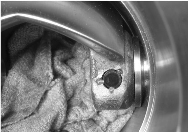
**Figure 43** 1 to 2" NPS Shaft Connection Stake Example
