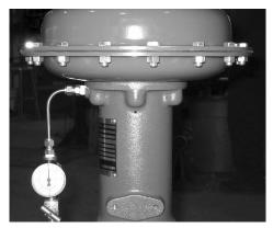
Figure 3 Needle Valve with Gauge setup
