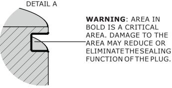
Figure 13 Two-Piece Plug Seal Ring Removal (Model 350)
