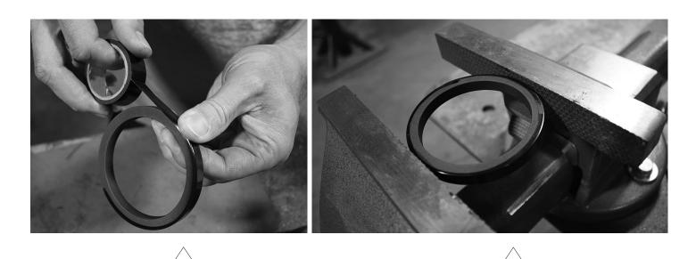
Figure 23 Model 351 Piston Ring Vise Break Method (Step 1)
