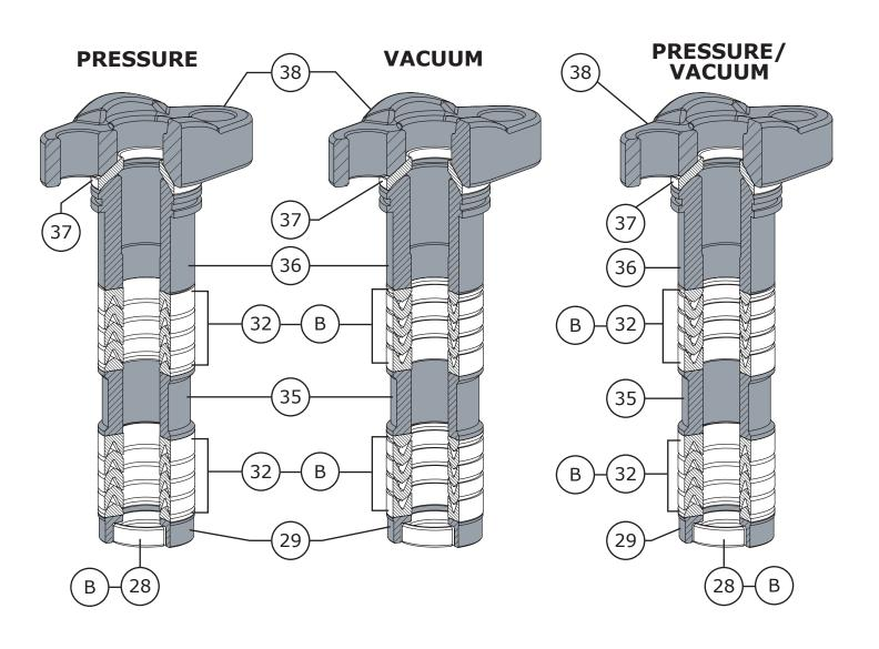
Figure 33 Double PTFE Packing Diagrams
