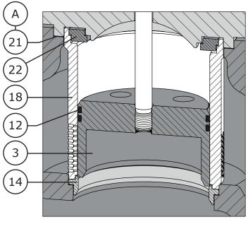
Figure 37 Load Ring Diagram (8 Inch Valve Assembly)
