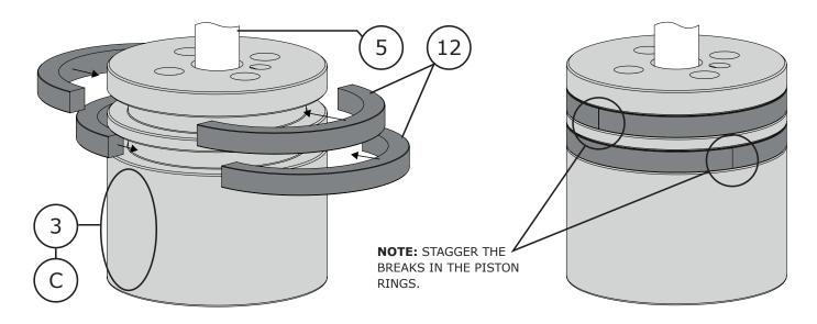
**NOTE:** APPLY GREASE TO ENTIRE OUTSIDE SURFACE OF PLUG.
