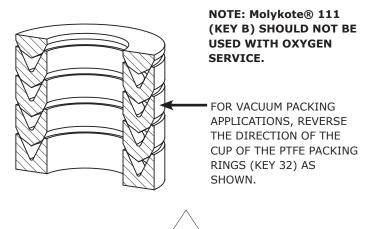
Figure 29 Single Style Packing Installation Diagram
