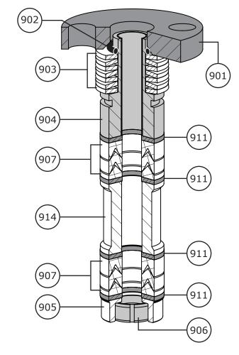
Figure 31 Graphite Packing Arrangement Diagram
