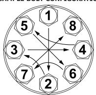
Figure 27 Bolt Tightening Pattern Diagram
