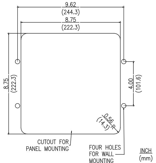
Figure 16 Mounting Details, Pipestand, Surface Panel
