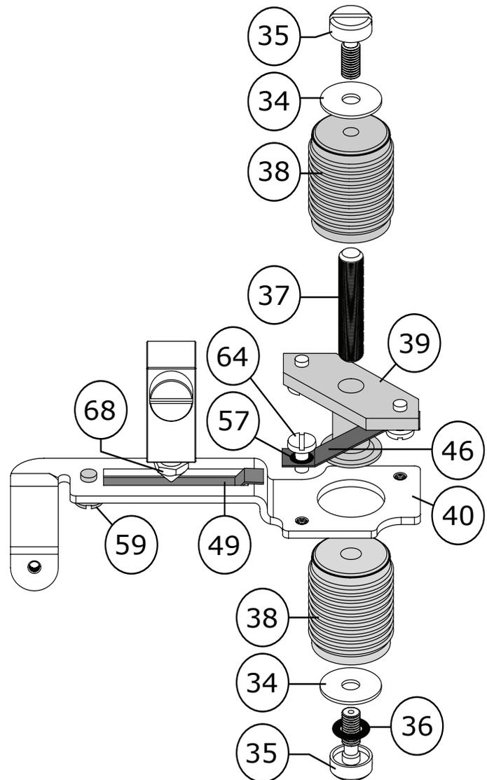
Figure 9 Bellows Sub-Assembly
