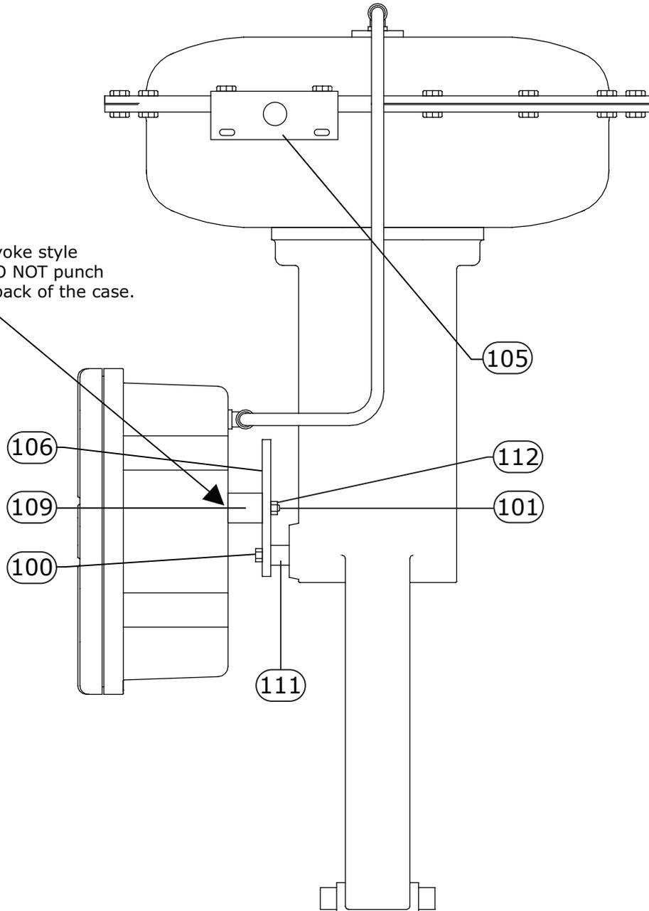
**Figure 17** *Mounting Details, Actuator Yoke*
