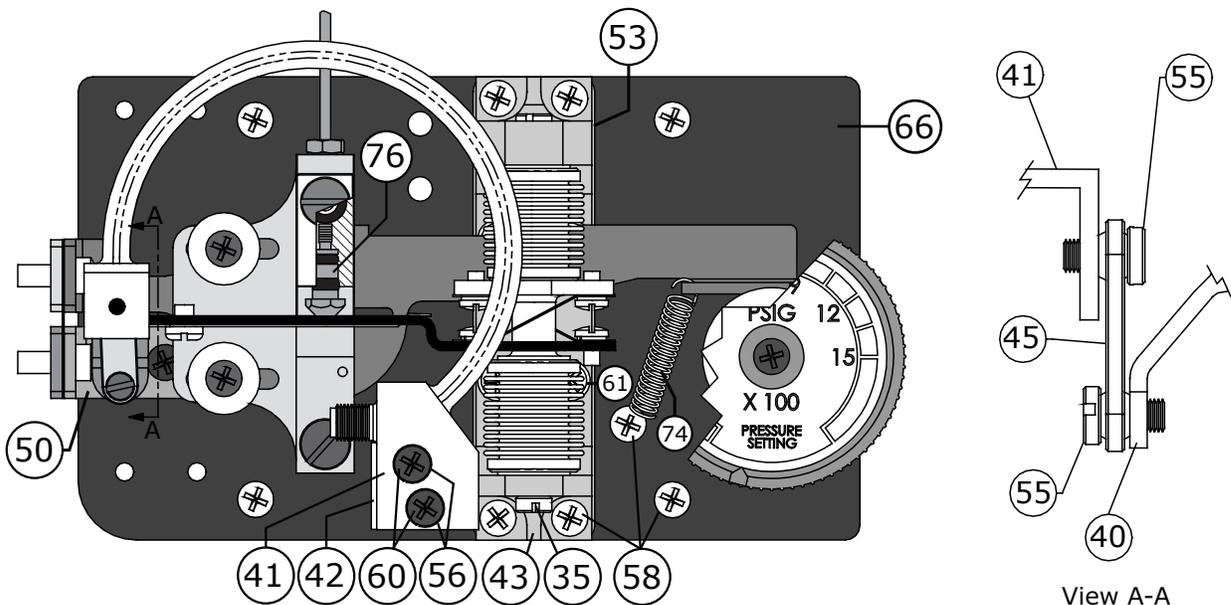
Figure 11 Old Style Mounting Base Sub-Assembly
