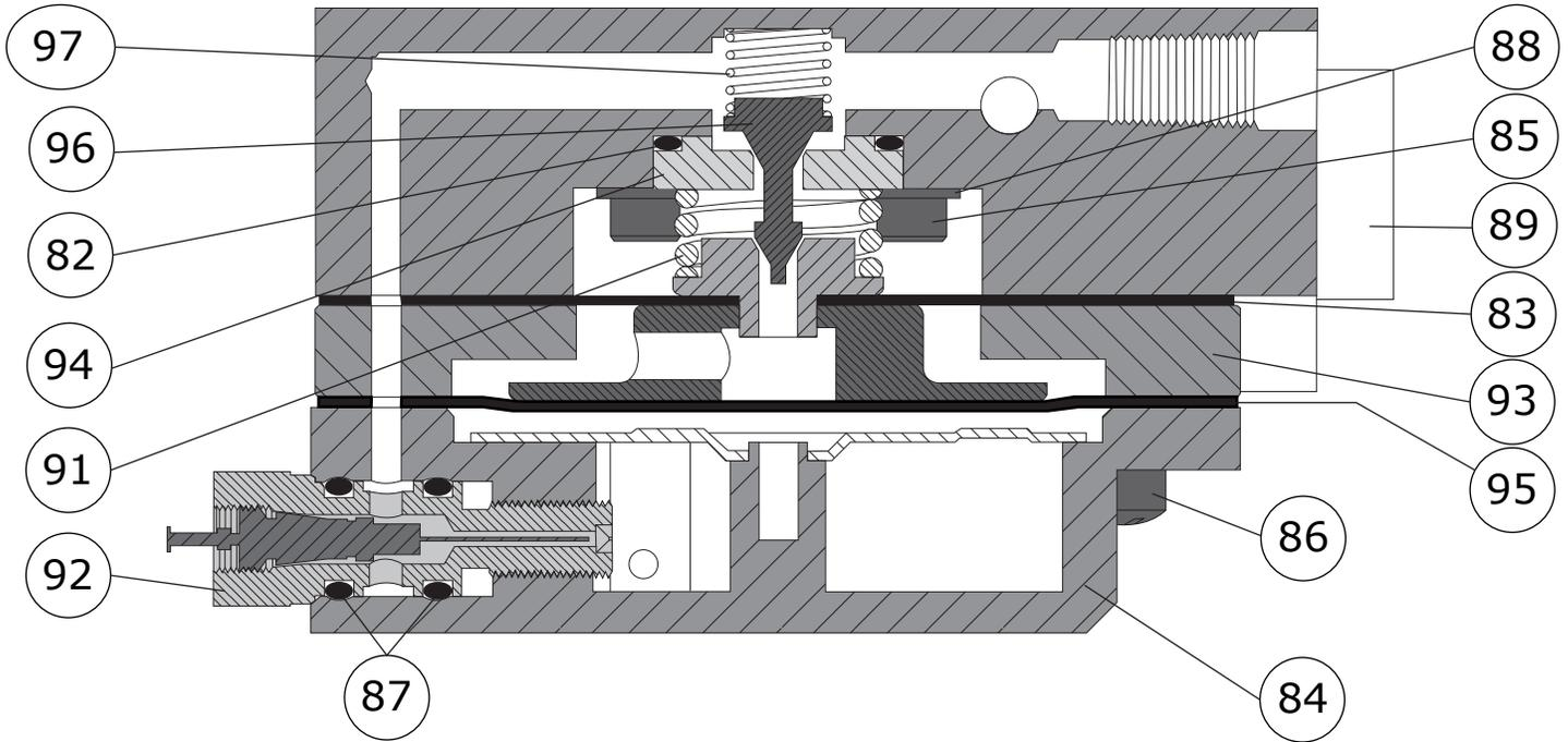
**Figure 7** New Style Relay Manifold Cross Section (Key 27)
