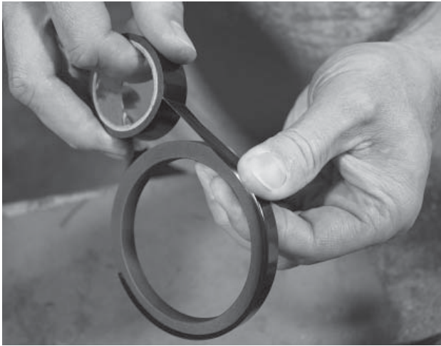
Figure 18 Piston Ring Assembly for Model 371 Valves (Step 1)
