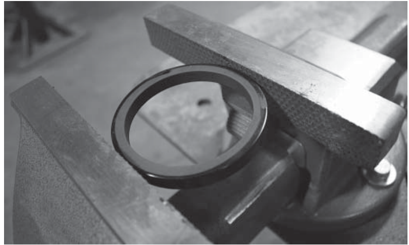
Figure 19 Piston Ring Assembly for Model 371 Valves (Step 2)
